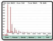
ing systems are susceptible to harmonic pollution. In fact, harmonics can cause small, almost imperceptible variations in performance that aggregate to affect significant long-term damage. Current harmonics generated by a source can pollute the entire power system without being affected itself. The Energy Platform captures detailed harmonics, interharmonics, and subharmonics in accordance with IEC 61000-4-7 and IEEE 519 to effectively troubleshoot the complex problems caused by these events.
