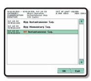
duration, and min/max while out of limits. Voltage and current waveform snapshots are also available and can be recorded on a periodic basis. Snapshots can be used to visually assess the quality of supply or used with Dran-View software. For more advanced power quality applications that require recording of waveshapes, transients, and other important power quality parameters, consider the PowerXplorer, PowerGuide, or PowerVisa from Dranetz
