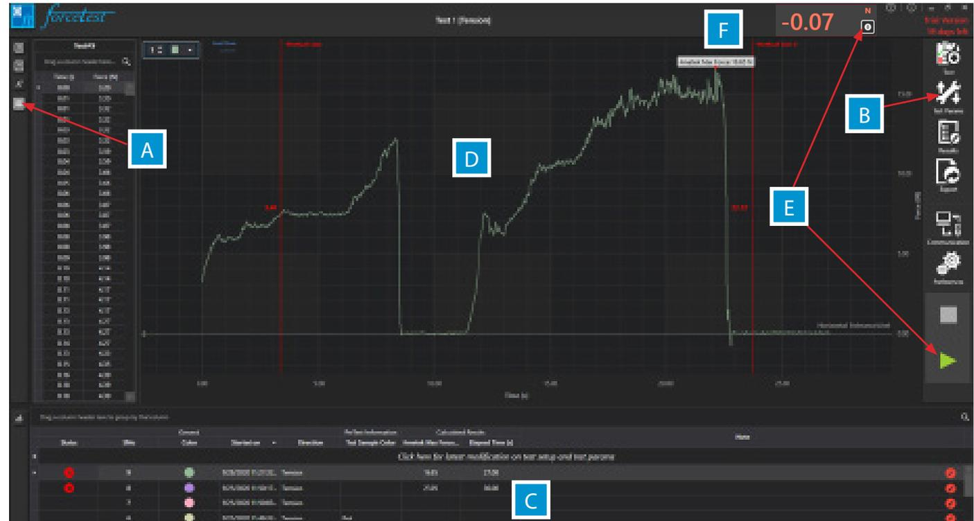
**D The Graph** The graph plots a running test run or the test run selected in the Test Record table. Once a test run is finished, the graph can be zoomed in and out using the CTRL key on the keyboard and a mouse wheel. When multiple test runs are selected in the Test Record table, the graph will overlay test runs to allow comparison between test runs.
