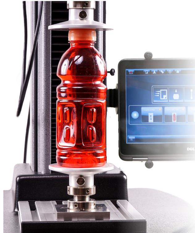
Conduct a quick test by simply entering the type of test, pre-load (if any) and limits.
