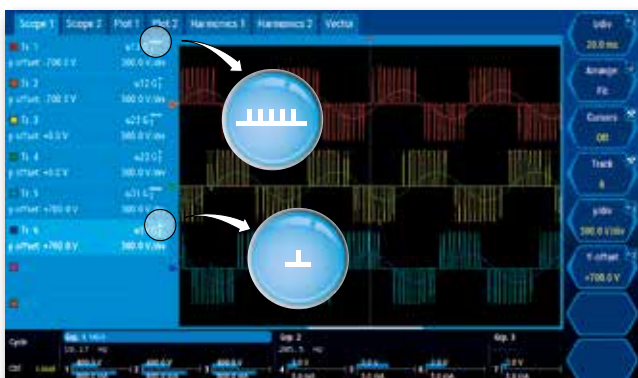
Scope display of the voltages at the converter output. The wideband values (noisy) show the PWM signal, the narrowband values (sinusoidal) are sinusoidal.
