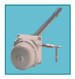
**Principle of Operation:** Direct-sensing insitu probe using zirconium oxide for net oxygen measurement.
