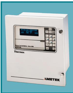
**Display:** Four-line x 20-character vacuum fluorescent. Displays combinations of oxygen, time and date, cell temperature, user programmable text, thermocouple mV or cell mV. Password protection, programmable pressure compensation and context-sensitive help are also provided.
