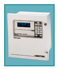
**Display:** Four-line x 20-character vacuum fluorescent. Displays combinations of oxygen, time and date, cell temperature, user-programmable text, thermocouple mV or cell mV. Password protection, programmable pressure compensation and context sensitive help are also provided.
