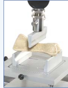
Bending test on bone-shaped dog chew
