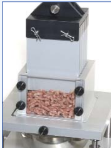
Minced meat firmness measurement using Kramer shear cell
