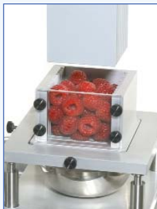
Ottawa forward extrusion of soft fruit
