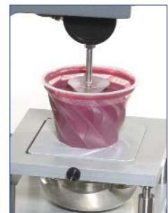
Penetrometer test using a cone probe
