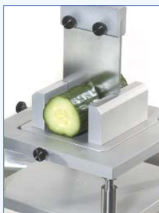
Cucumber cutting force using Warner-Bratzler shear jig
