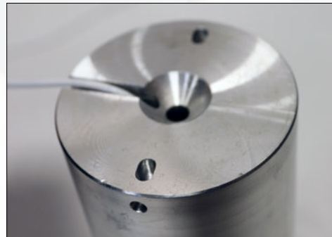
STS-102 A 035 sensor in an insert.
