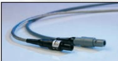
The well-reputed JOFRA STS reference sensors as well as the new DLC reference sensor are all mounted with intelligent plugs containing all individual information regarding the sensor.
