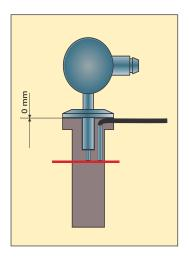
Below you see the custom insert and STS-102 A reference sensor placed in a JOFRA ATC-156 B dry-block calibrator. On the right, the sanitary sensor has been fitted into the insert and is ready for calibration. Note that the design makes room for the reference sensor cable.
