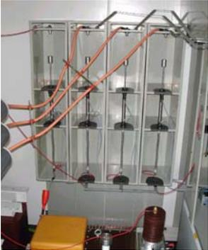
**Pneumatic Switching Units (PSU)**
