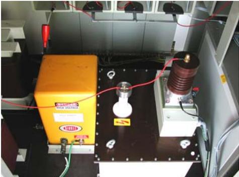
**AC & DC High Voltage Unit (18kV & 70kV)**
