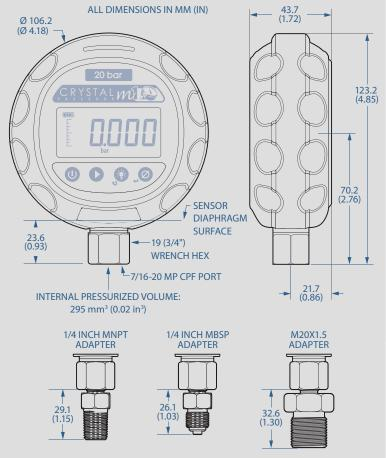
ADDITIONAL SENSOR LENGTH WITH OPTIONAL FITTING ADAPTERS
