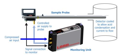
person and no special skill to take the readings. The operator has to adjust the air supply and obtain a steady current flow on the display.
